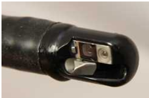
Figure 1: ERCP 用内視鏡の先端 (拡大)
